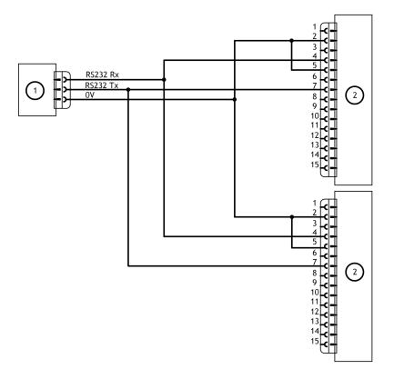
1. RS485 interface on control equipment 2. pump logic interface
